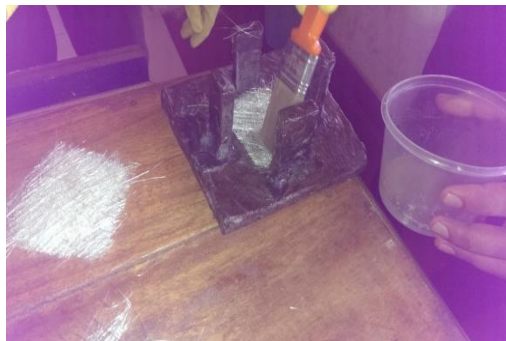
Figure 1: Shows Hand layup Method
