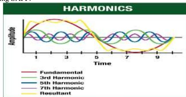
Figure 1: The fundamental wave, Resultant wave, 3<sup>rd</sup>, 7<sup>th</sup> & 5<sup>th</sup> harmonics in system.
