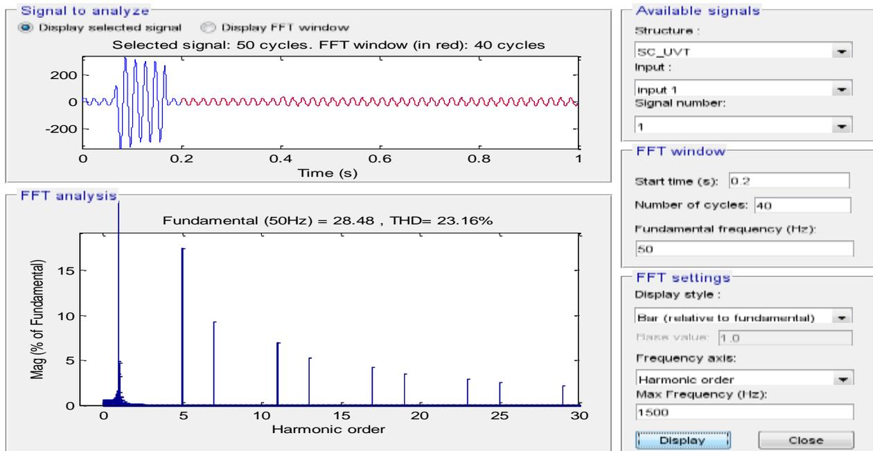
Figure 10: Harmonics produced in source current when filter was not connected to the system. In this case the THD of the system is 23.78%. same as THD present in load current .
