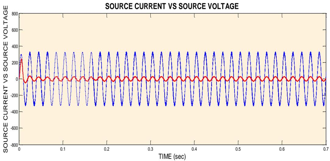
Figure 7: Source voltage and source current, in the absence of filter.
