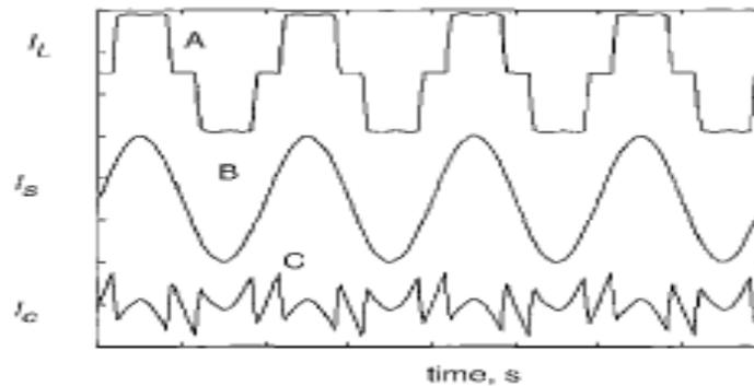
**Figure 3: Shape of load current, source current and compensating current**
