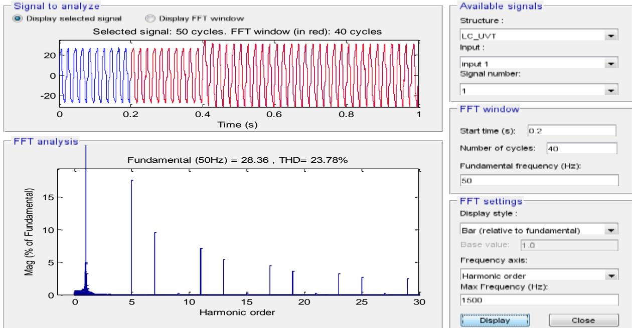
Figure 9: FFT analysis done to find Total Harmonic distortions in load current. Clearly the THD of load current is 23.78%
