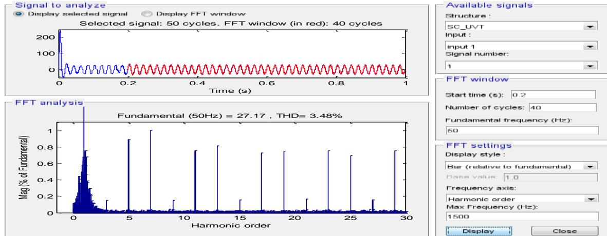
Figure 11 THD in source current after performing the FFT analysis, when the filter is connected to the system. In this case the harmonics in the system gets reduced and it is clear in the figure that the THD is reduced from 23.78% to 3.48%, which is less than 5% as per IEEE-519 standards.
