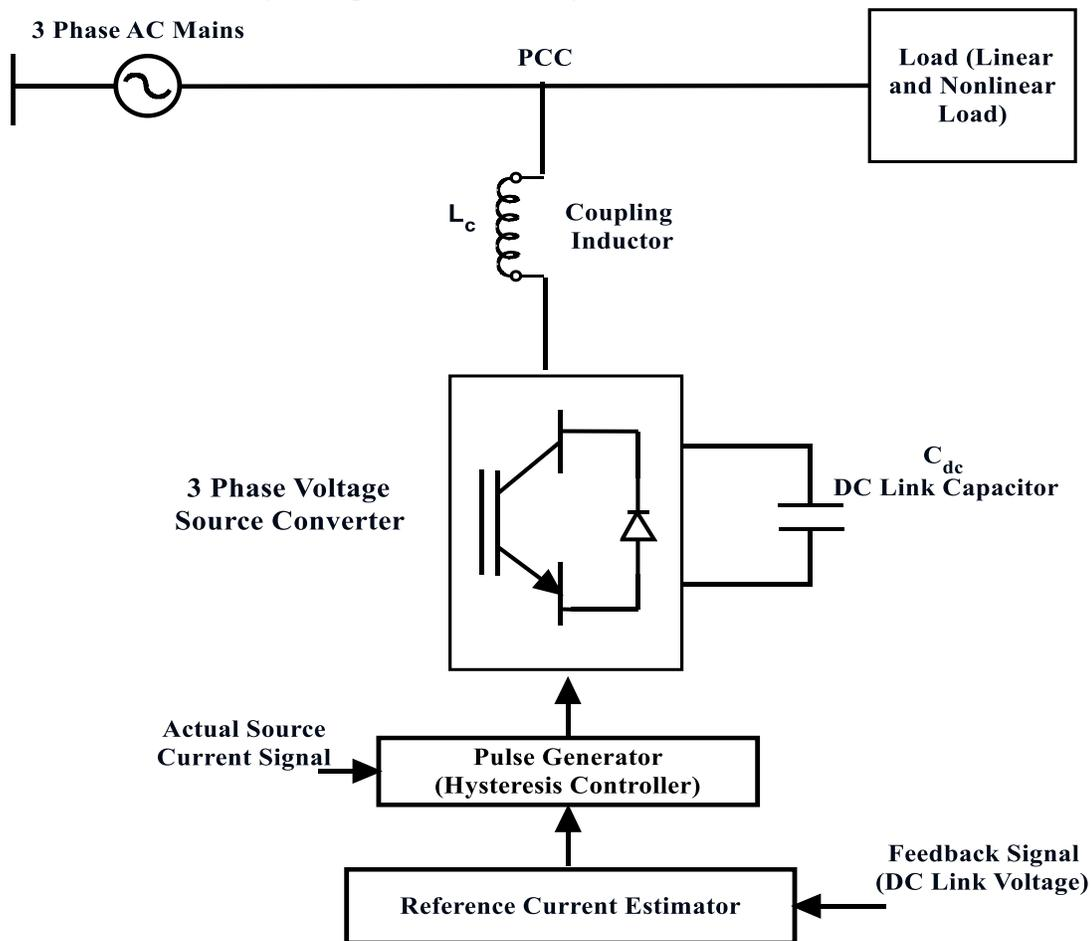
Figure 4: The schematic diagram of SAPF.
