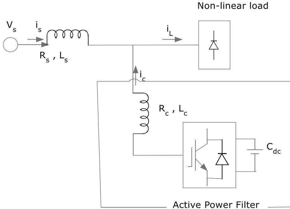
**Figure 2: Compensation principle of SAPF.**
