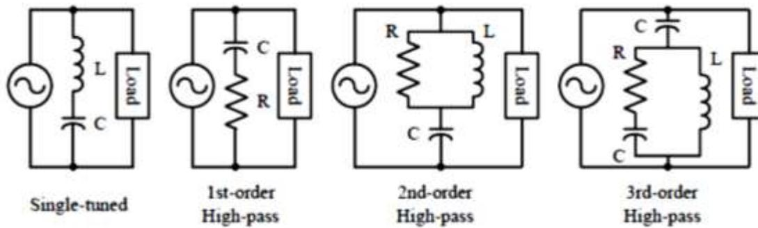
Figure. 1: Common types of passive filters and their configurations
