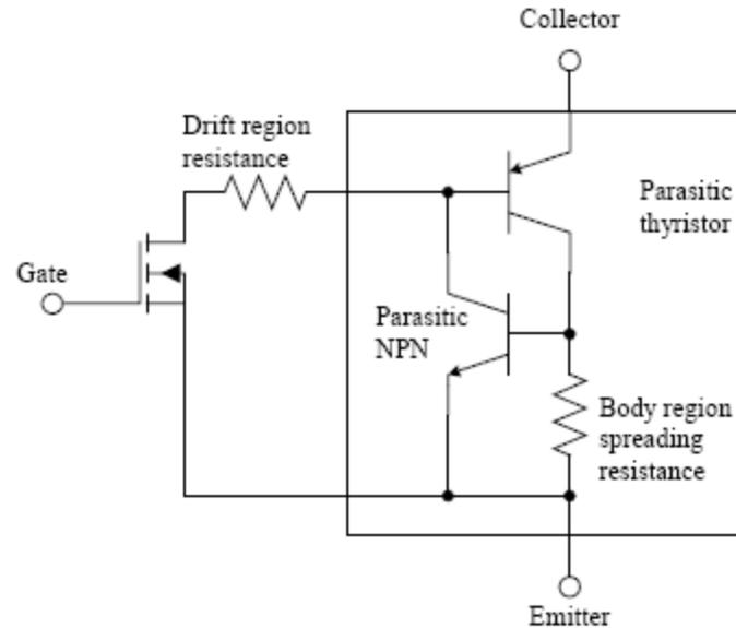
Figure 2:Equivalent Circuit of IGBT
