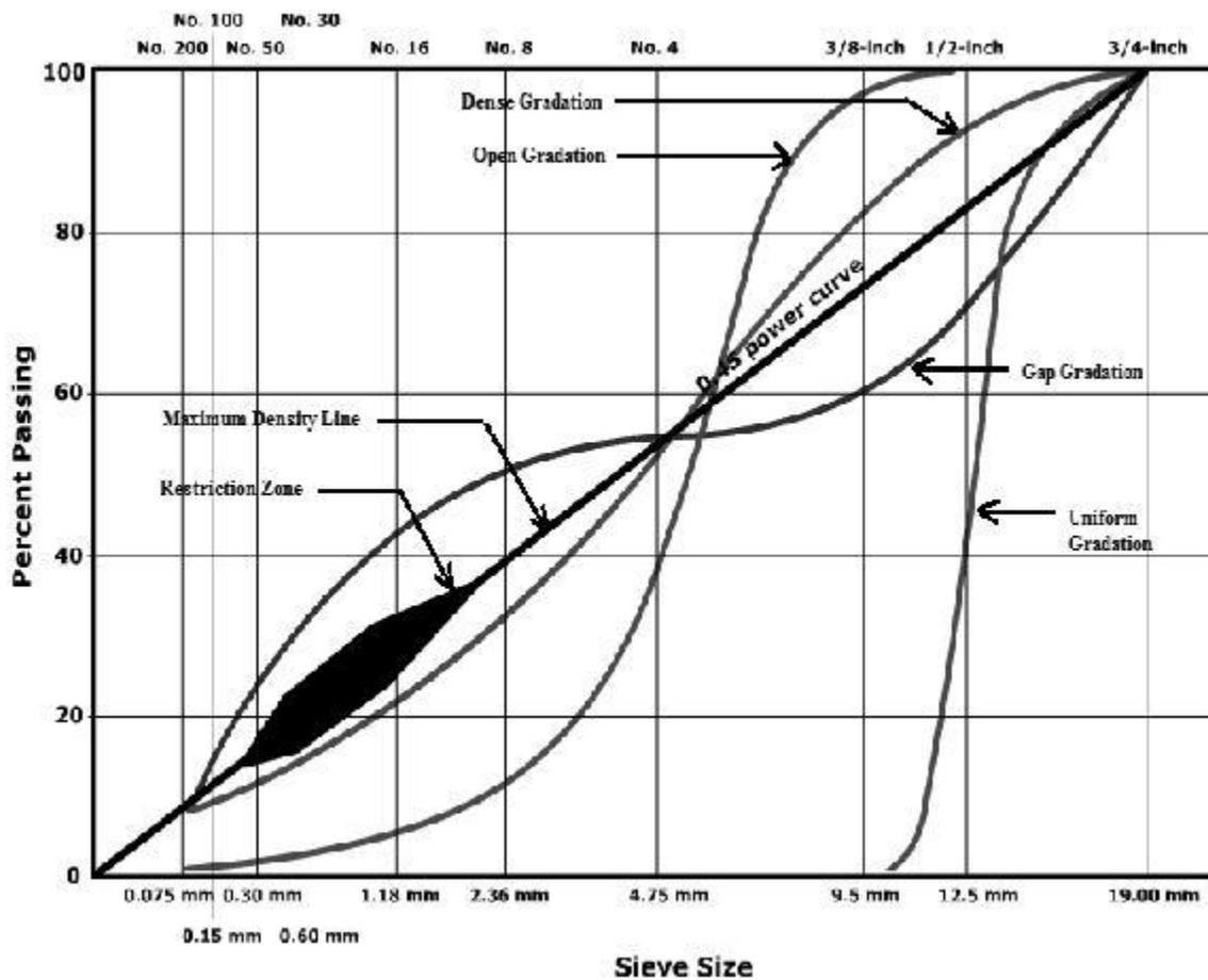
Figure 3.20 FHWA gradation graph showing representative gradations
