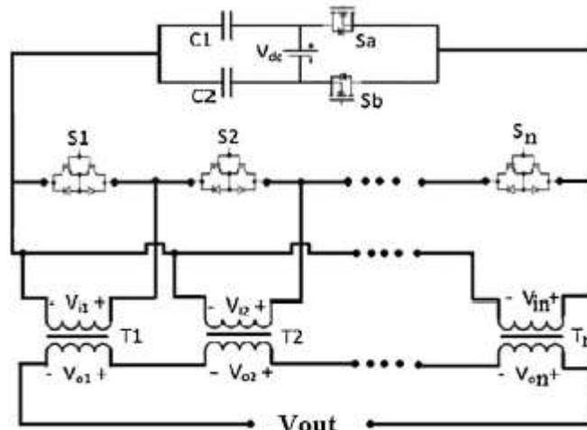
Figure 5: proposed multi-level inverter
