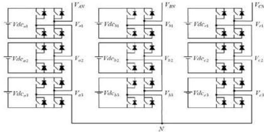
Figure 3: Cascade Multilevel converter
