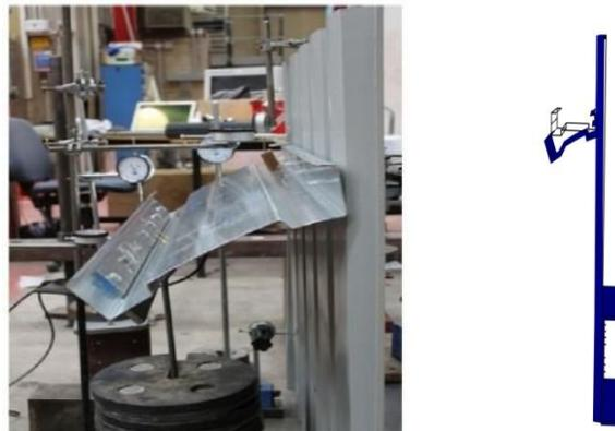
Figure 2. Experimental deformation for  $\Sigma 20012FU$  compared to the FE model
