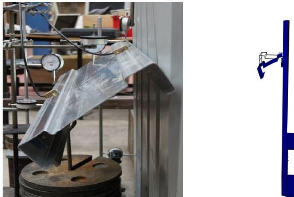
Figure 3. Experimental deformation for  $\Sigma 20012FD$  compared to the FE model
