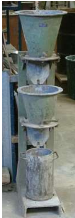
Figure 5.1 – Apparatus Used to Conduct the Compacting Factor Test
