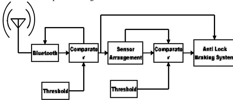
Fig. 1. Signal Flow Diagram of Bluetooth Enabled Collision
