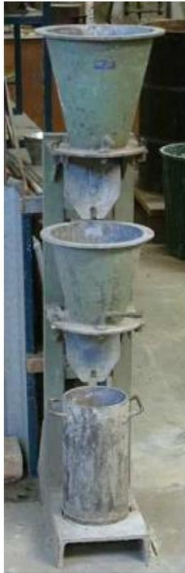
FigureNo.02 – Apparatus Used to Conduct the Compacting Factor Test
