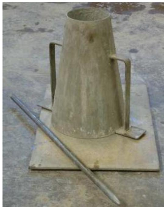
Figure No. 01 – Equipment Required to Conduct a Slump Test
