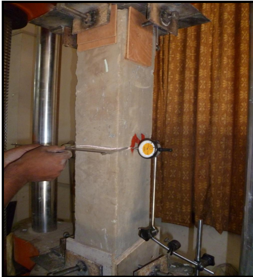
Fig 2 :Compressive Strength Test on Columns
