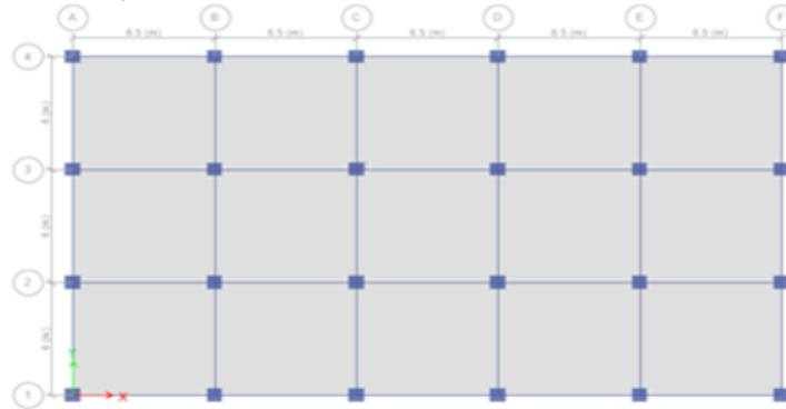
Fig.1 Model 1 – Floor plan of the structure without shear wall.
