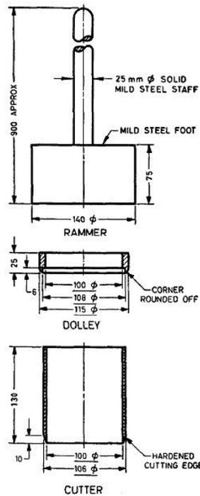
Fig. 2. Core Cutter Apparatus
