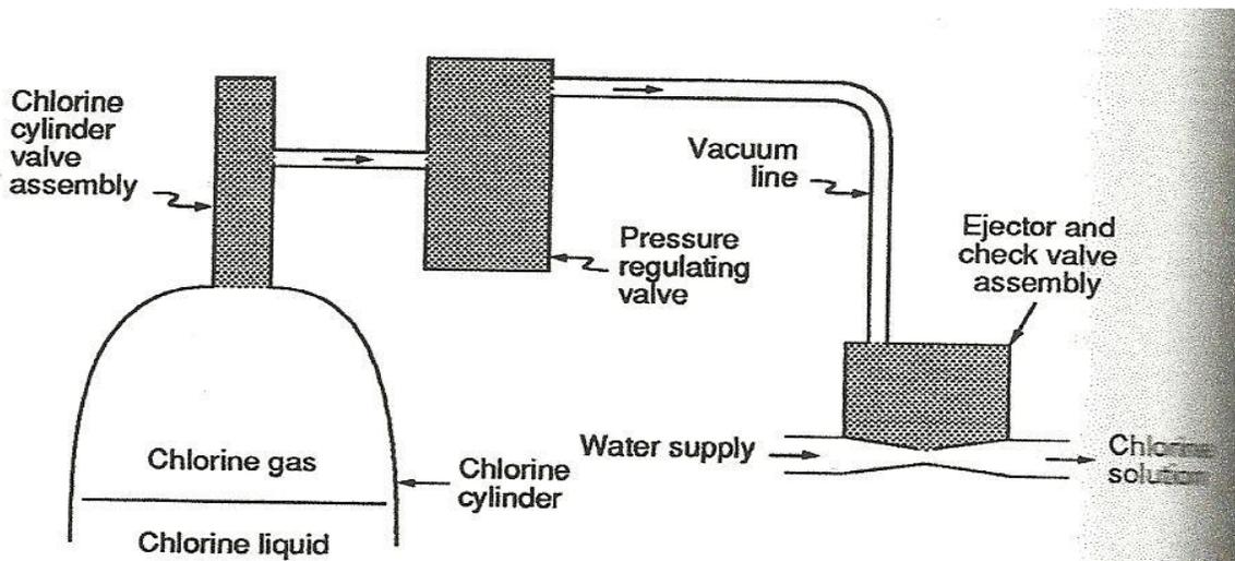
Fig No.01 Chlorination Flow Diagram
