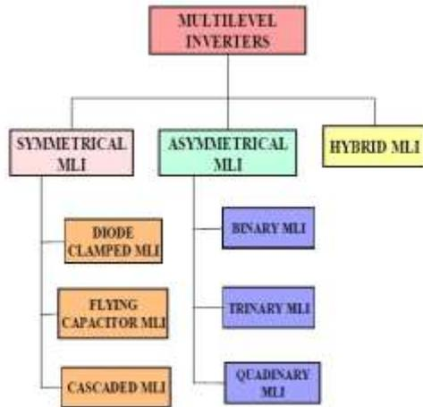
Fig.1: Types of multilevel Inverters
