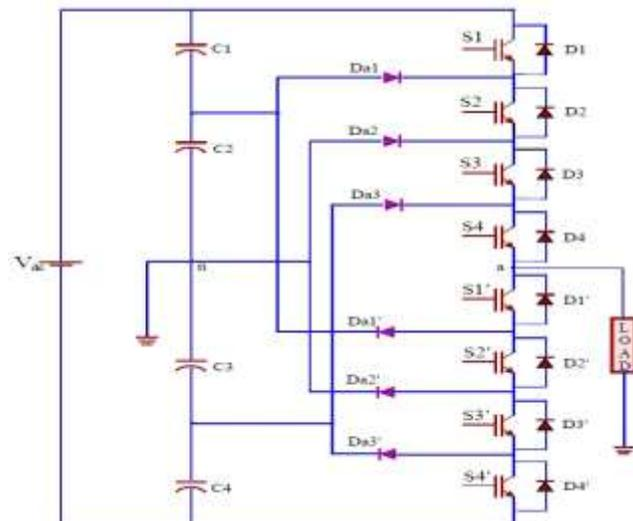
Fig.2: Five level diode clamped multilevel inverter
