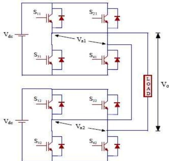
Fig.4: Five level cascaded multilevel inverter
